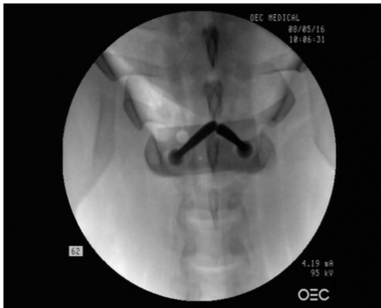
Figure 4.3.3 Fluoroscope Image of accelerometer block mount screw placement and securement at the T1 location for the 50 th percentile male PSE
