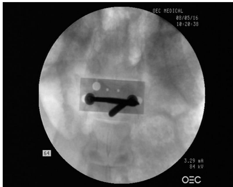
Figure 4.3.5 Fluoroscope Image of accelerometer block mount screw placement and securement at the L6 location for the 50 th percentile PSE
