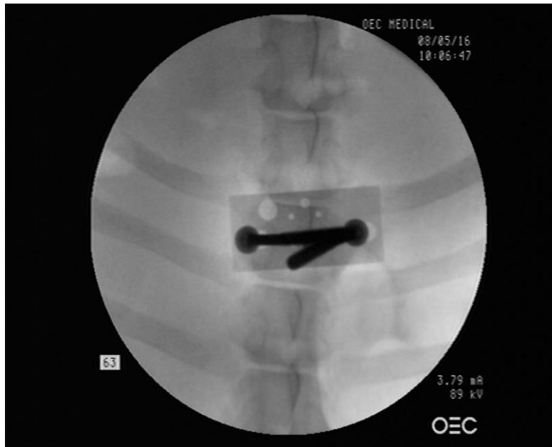
Figure 4.3.4 Fluoroscope Image of accelerometer block mount screw placement and securement at the T14 location for the 50 th percentile male PSE
