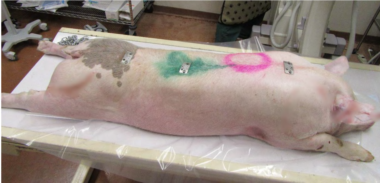
Figure 4.3.6 Overall view of the placement of the accelerometer block mounts relative to each other for the 50 th percentile male PSE
